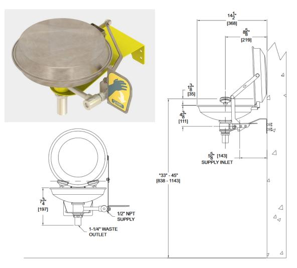
Model S0440-CS1 is our wall mounted eye/face wash with stainless steel bowl and clam shell cover. Complete with plastic eye wash spray heads and dust covers. Compliant to ANSI Z358.1 standards and includes safety sign and weekly testing card.
